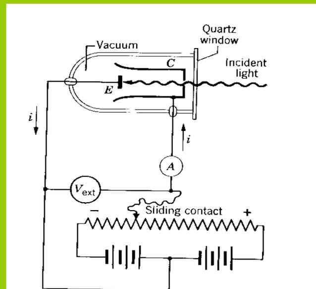
An apparatus used to study the photoelectric effect. The collected photoelectrons move in a direction opposite to that indicated by the conventional current arrows.
