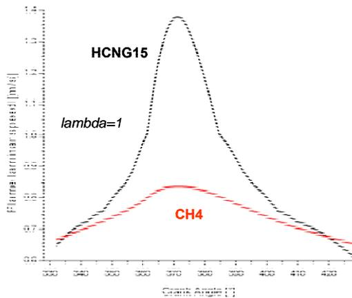
Methane has a slow flame speed while hydrogen has a flame speed about eight times higher; when the air/fuel ratio ( $\lambda$ ) is much higher than for the stoichiometric condition the combustion of methane is not as stable as with HCNG.
