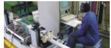
Continuous testing of superconductor cables during production
