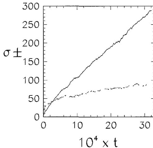
Fig. 15. — Dependence of second moments on time for the Lloyd model with  $\nu = 3$ ,  $k = 0.2$ ,  $U = 2$ ; upper curve is  $\sigma_+$ , lower is  $\sigma_-$ . At  $t = 0$  both particles are at  $n = n' = 0$ . Basis is  $128 < n, n' < 128$ . For  $U = 0$  one has  $\sigma_+ \approx 2$ .
