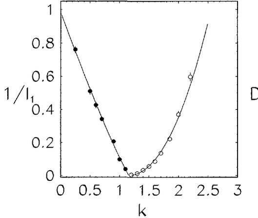
Fig. 9. — One-particle Anderson transition in the model (3) with  $V$  from (10)  $\nu = 3$ ,  $\epsilon = 0.9$  as a function of hopping  $k$ . Critical point  $k_{\text{cr}} \approx 1.15$ . One particle localization lengths ( $l_1$ ) and diffusion coefficient ( $D$ ) are evaluated from the fitting of probability distribution. Error bars indicate the standard deviation for ensemble of 100 (localized) and 10 (diffusive) different random realizations. Lines are drawn to fit an eye.
