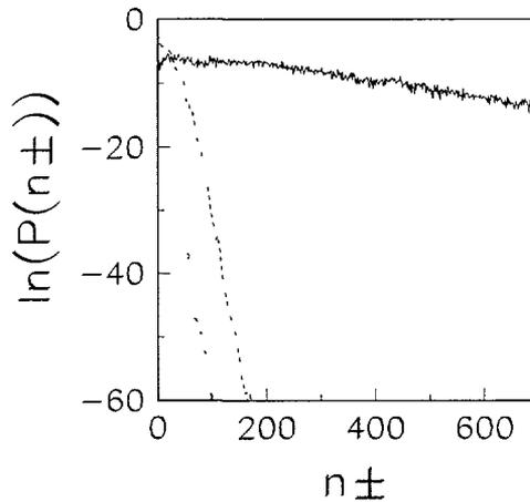
Fig. 11. — Probability distribution at  $t = 1.6 \times 10^6$  as a function of  $n_{\pm} = 2^{-1/2}(n \pm n')$  for the case of Figure 10:  $P_+(n_+)$  (full line);  $P_-(n_-)$  (dashed); dotted line is the distribution  $P_+(n_+)$  for  $U = 0$ .
